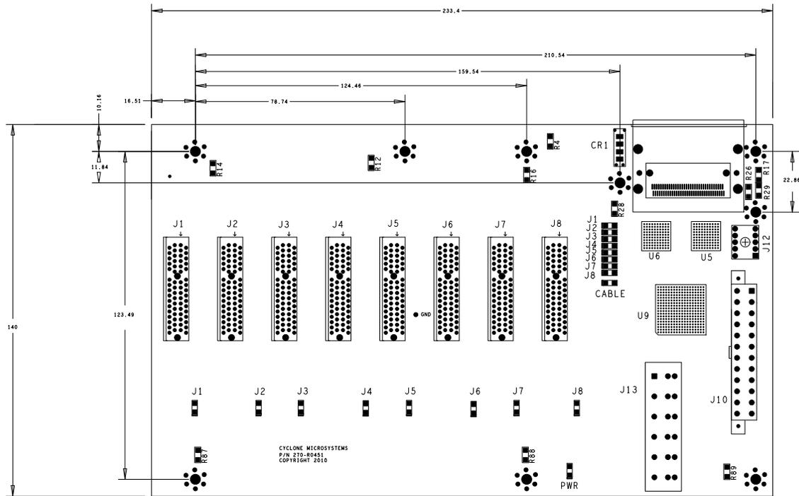
**Figure 5-1. PCIe-451 Physical Configuration**
