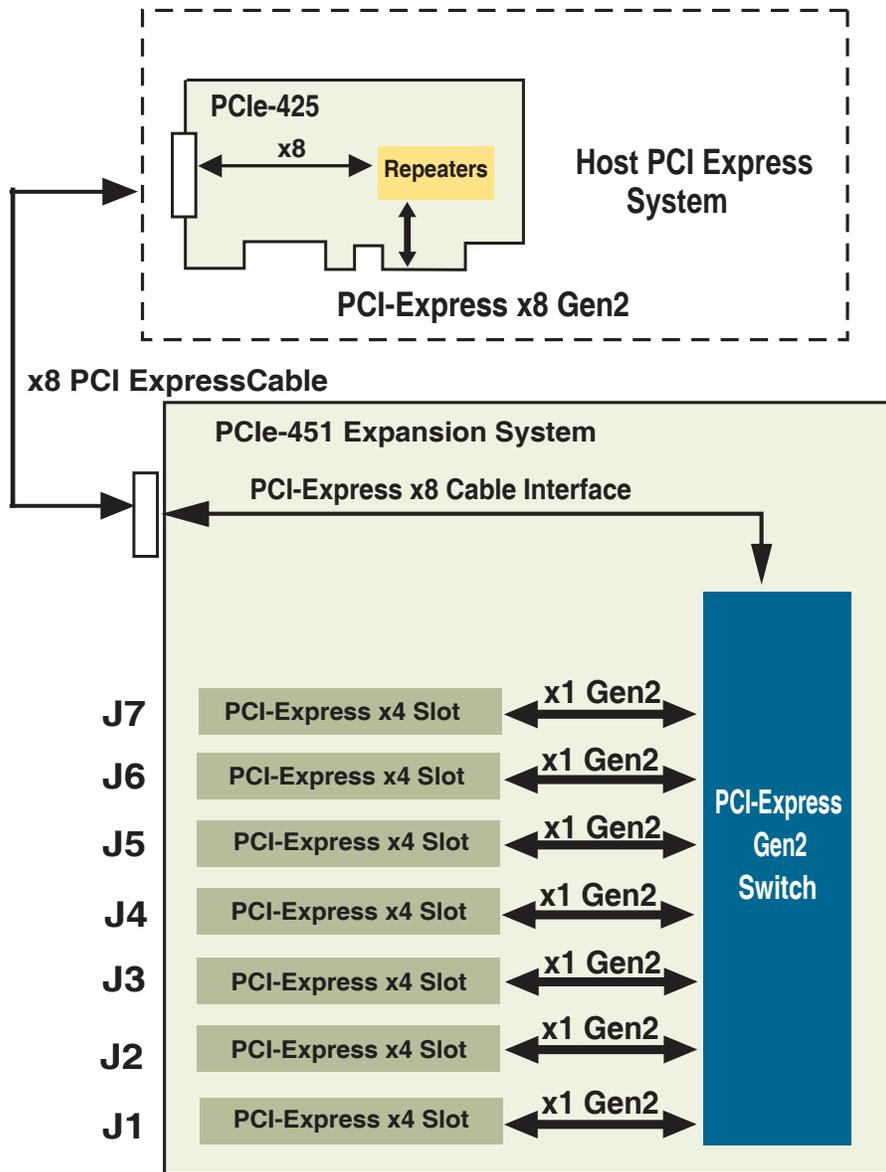
Figure 1-1. 600-2708 Block Diagram
