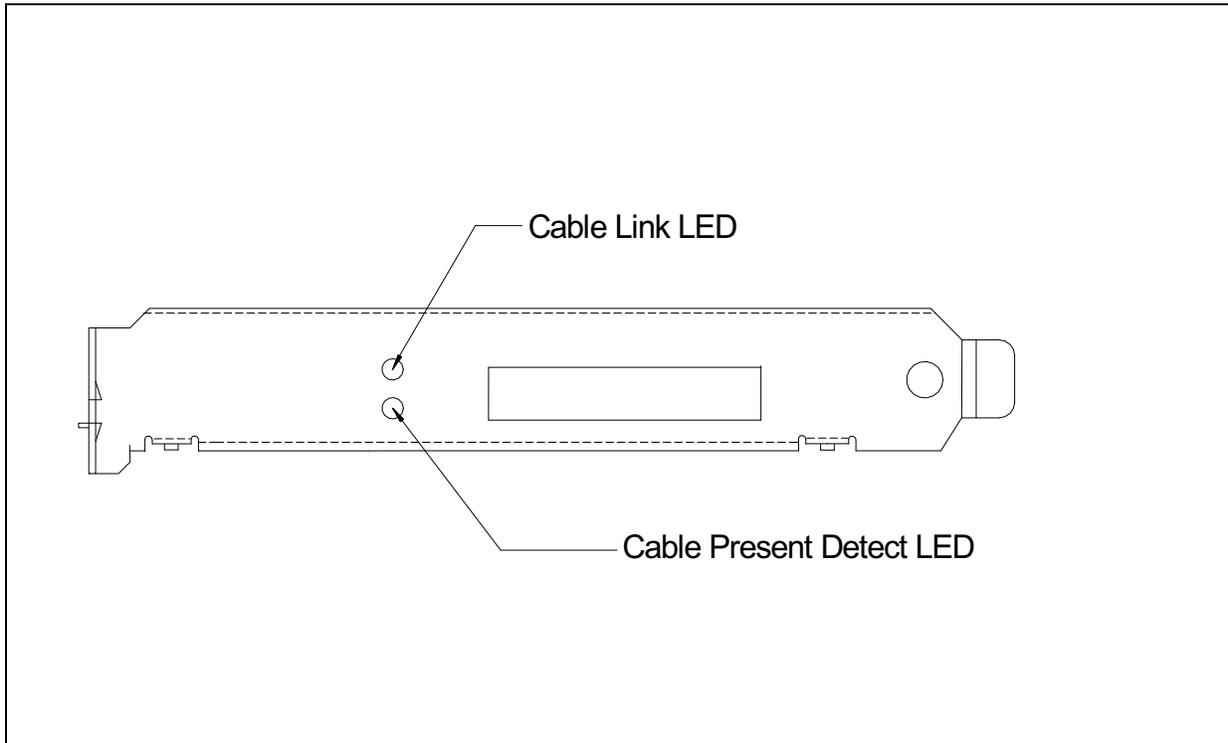
Figure 5-2. PCIe-425 Front Panel
